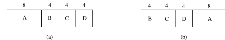
Figure 2-40. An example of shortest job first scheduling, (a) Running four jobs in the original order, (b) Running them in shortest job first order.
